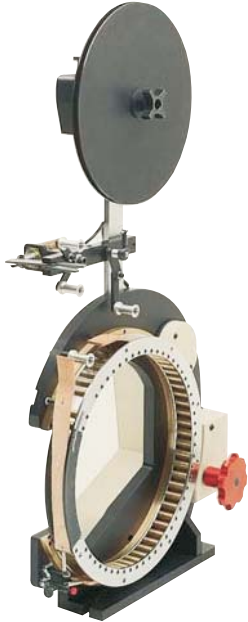
14" Taping and Shielding Head Maximum Coil O.D.: 17.0" (431.3 mm) Minimum Coil O.D.: 3.0" (76.2 mm) Minimum Coil I.D.: 2.0" (50.8 mm) Maximum Coil Height: 6.0" (152.4 mm) Tape Widths: 5/16", 3/8", 1/2", 5/8", 3/4", 1" (8 mm, 10 mm, 12 mm, 15 mm, 19 mm, 25 mm)
