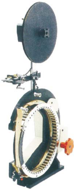
14" Taping and Shielding Head Maximum Coil O.D.: 10.0" (254.0 mm) Minimum Coil O.D.: 3.0" (76.2 mm) Minimum Coil I.D.: 2.0" (50.8 mm) Maximum Coil Height: 3.5" (88.9 mm) Tape Widths: 5/16", 3/8", 1/2", 5/8", 3/4", 1" (8 mm, 10 mm, 12 mm, 15 mm, 19 mm, 25 mm)
