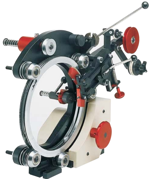
12" Gear Head Maximum Coil O.D.: 15.0" (381.0 mm) Minimum Coil O.D.: 3.0" (76.1 mm) Minimum Coil I.D.: 1.625" (41.2 mm) Maximum Coil Height: 6.0" (152.4 mm) Wire Size: #8 ?#20 AWG (3.25 ?0.81 mm)
